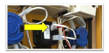
Hour Meter Connection for Orange Wire
