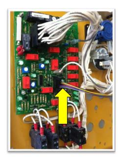
Controller Board with 10-pin Cable
