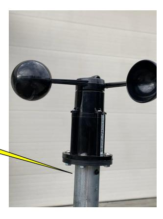
Use the small screw as a retainer. It does not need to be tight on the mast.
