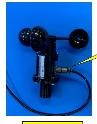
Attach cable to Wind Sensor
