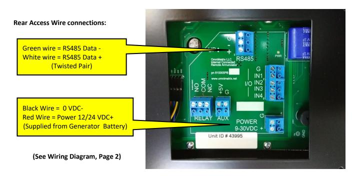
**Power On** instantly occurs when the 12vdc power source is connected to the Annunciator and made active. There is no power on button.
