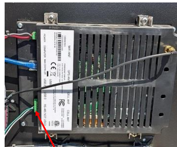
PowerZone Modbus RS485 connection
