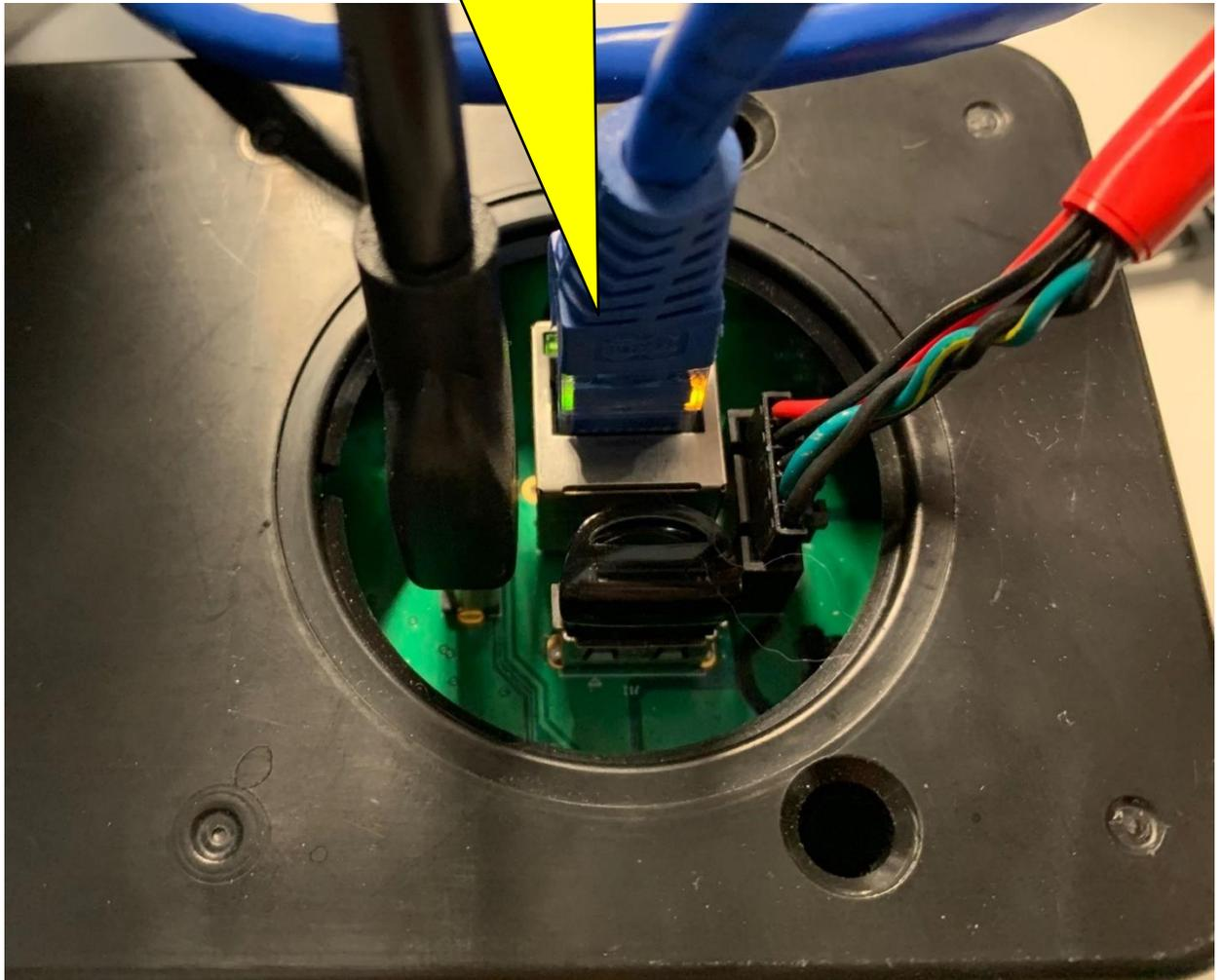
Attach the OMNI power wires, Red and Black, to generator Battery + and – respectively.
