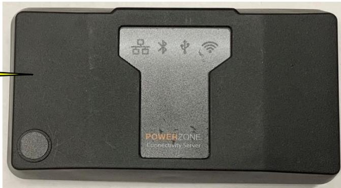
On the bottom side of the Connectivity Server is an RJ45 connector in the center. Plug the OMNI CAT5 cable into this RJ45.
