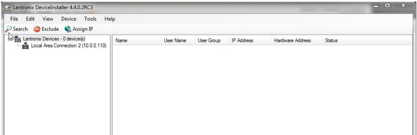
4. Click on the SEARCH icon and the DeviceInstaller should find the Lantronix device on the network. It will be named "XDirect-IAP", and if it has found its way onto your network via DHCP, you will see its current IP Address and MAC Address, as shown below.
