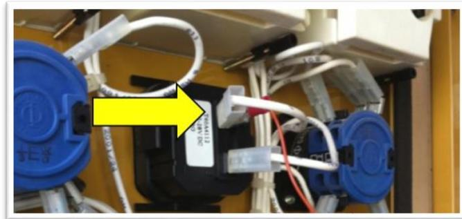
Hour Meter Connection for Orange Wire
