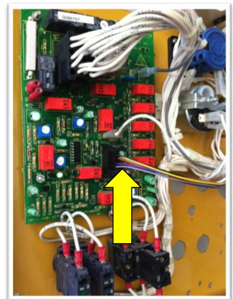
Controller Board with 10-pin Cable
