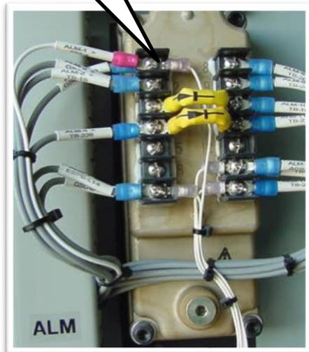
White/Gray wire to ALM on terminal strip and 20K OHM Resistor wire from ALM to Battery +.
