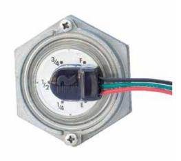
A magnetic drive allows a signal from the float mechanism inside the tank to be transmitted through a solid, non-magnetic bulkhead without the necessity of dynamic seals or pressure-type conductors.
