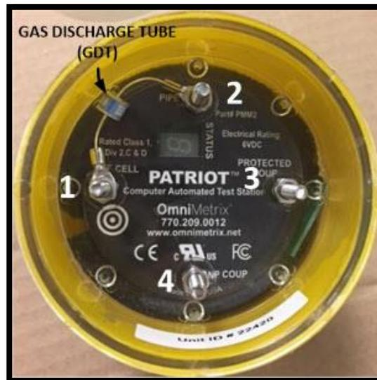
The Patriot has a 75V Gas Discharge Tube (GDT) installed to prevent damage to the electronic circuitry due to voltage spikes occurring during interruption operations. The GDT should remain in place during and after installation.
